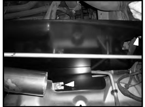
12. Install the rubber coupler to the throttle body and intake two with two large clamps.
