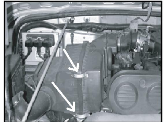
7. Remove 10 mm Nut holding the air box, and remove air box.
